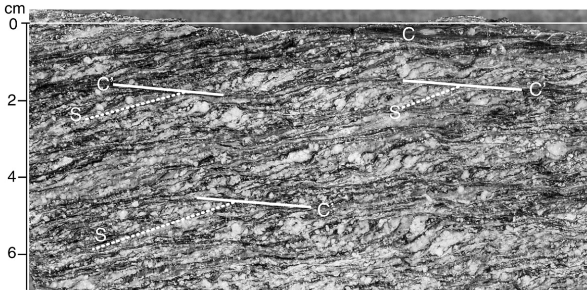
Fig. 3. Close-up near the shear zone center showing S–C–C' fabric. Scale corresponds to Fig. 2 and this picture is located at the top of Fig. 2.
